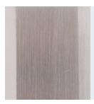
Characterized by finer grit lines and higher reflectivity than #4 finish. Improved product release, as well as cleanability. 25 Ra target.
