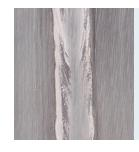
**BUFF** Minimal removal of weld material. Welds are not ground flush and may contain crevices, ripples, and irregularities in the remaining weld material.
