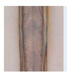
AS-IS Quality welds are to remain as deposited with no grinding.
