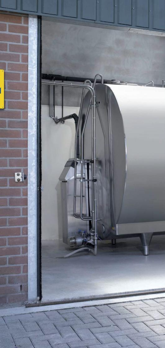
IDEALLY, THE CLEANING WATER TEMPERATURE SHOULD CONSTANTLY BE AROUND 45°C. IF NECESSARY, THE MUELLER INLINE HEATER HEATS UP THE CLEANING WATER DURING THE CLEANING PROCESS, TO ENSURE THE PERFECT TEMPERATURE AT ALL TIMES.
