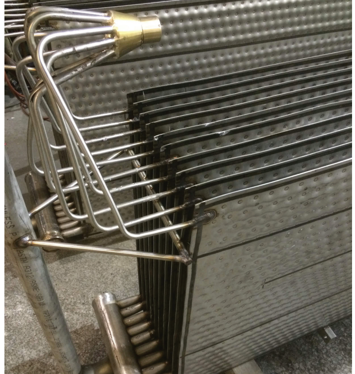
Energy recovery banks for heat recovery from hot gas.
